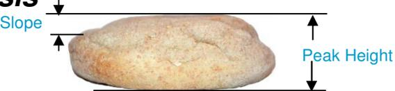
**Profile height calculations** are based on hundreds of individual height values gathered on every product, which leads to a measurement accuracy of  $\pm 0.5\text{mm}$ . **Mean Height** is another common measurement applied to english muffins.
