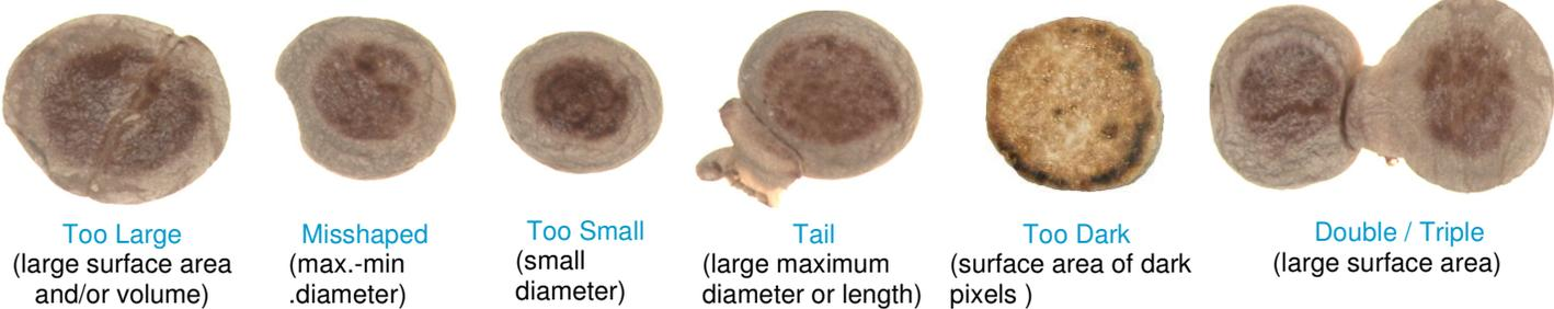
Only common examples have been pictured. There are many standard measurements that can be used, individually or combined within formulae, to qualify your product. **All visible product characteristics and faults can be quantified.**
